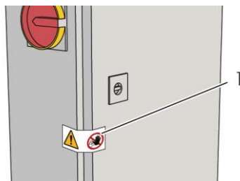
Fig. 66: Seal on switch cabinet
